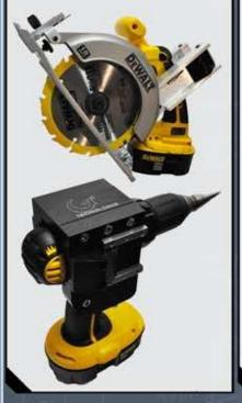
The Rotation Activated Tool System (RATS) was developed by Gl<sup>2</sup> Technologies to give robot operators the ability to use power tools, regardless of their robotic platform.
