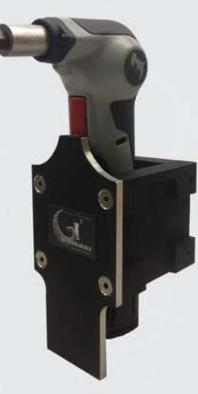
The device can break multiple windows on a single charge. There are NO electrical connections needed between the tool and the robot. Simply pick up the tool and push it up against the window you intend to break. This device only requires 2 lbs. of force to activate, making it ideal for smaller robotic platforms.
